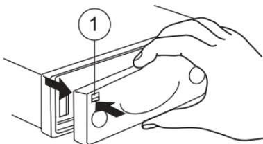
⇒ First pull the operating panel forward and then slide it to the left to remove it.
